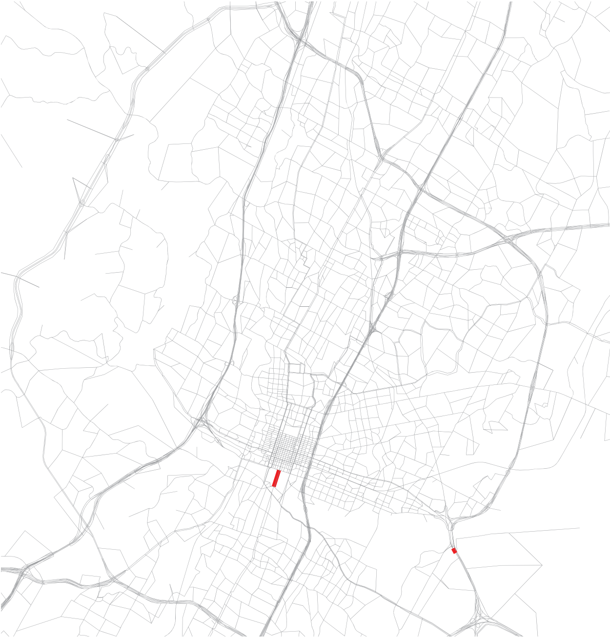
Figure 3: STA-Q 2015 Model Afternoon Peak Period Volume-to-Capacity Ratio Exceeding 1.1 (RED)
