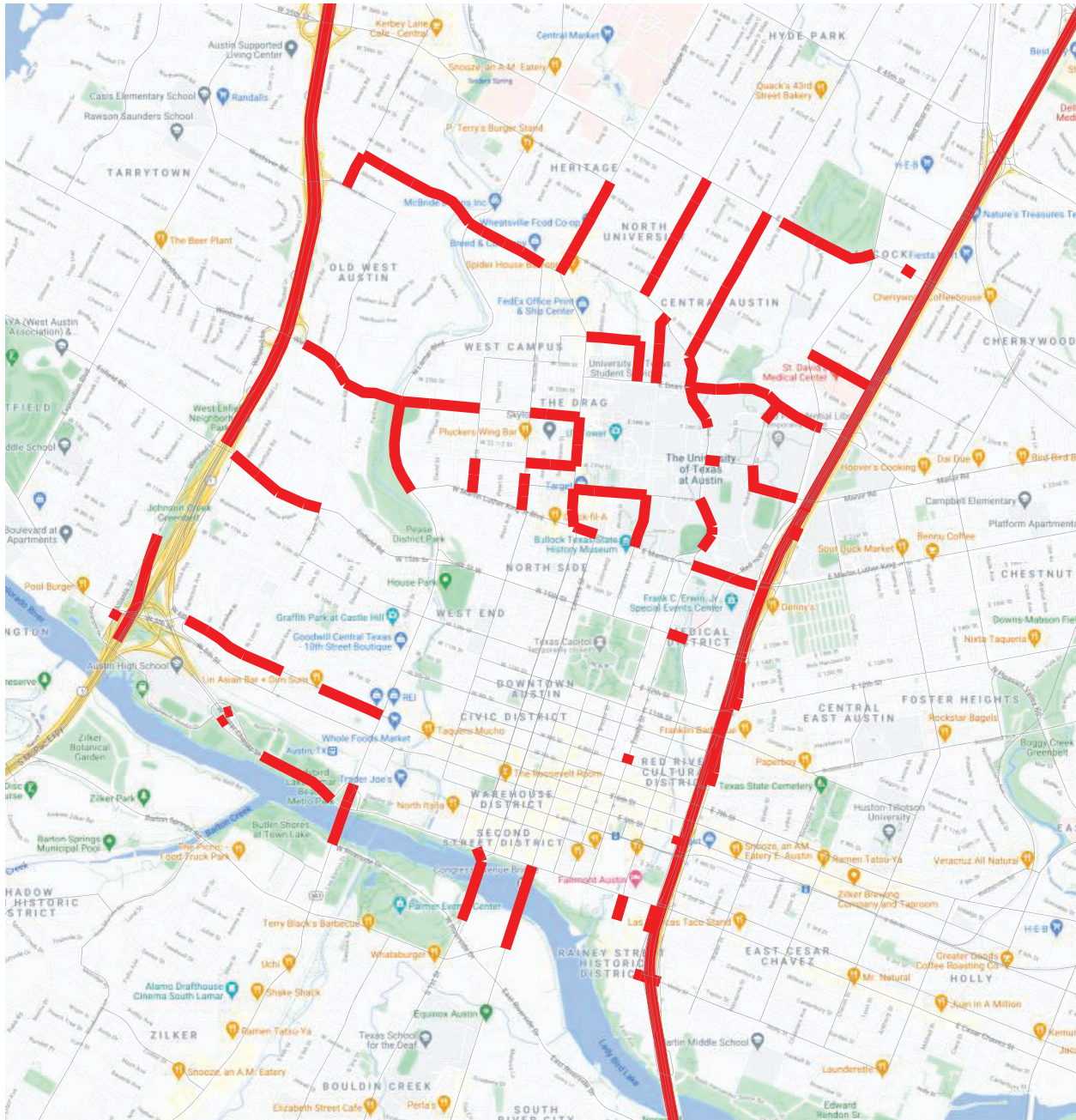
Figure 11: STA-Q Model 2045 Afternoon Peak Period Volume-to-Capacity Ratio Exceeding 1.1 Downtown Austin (RED)
