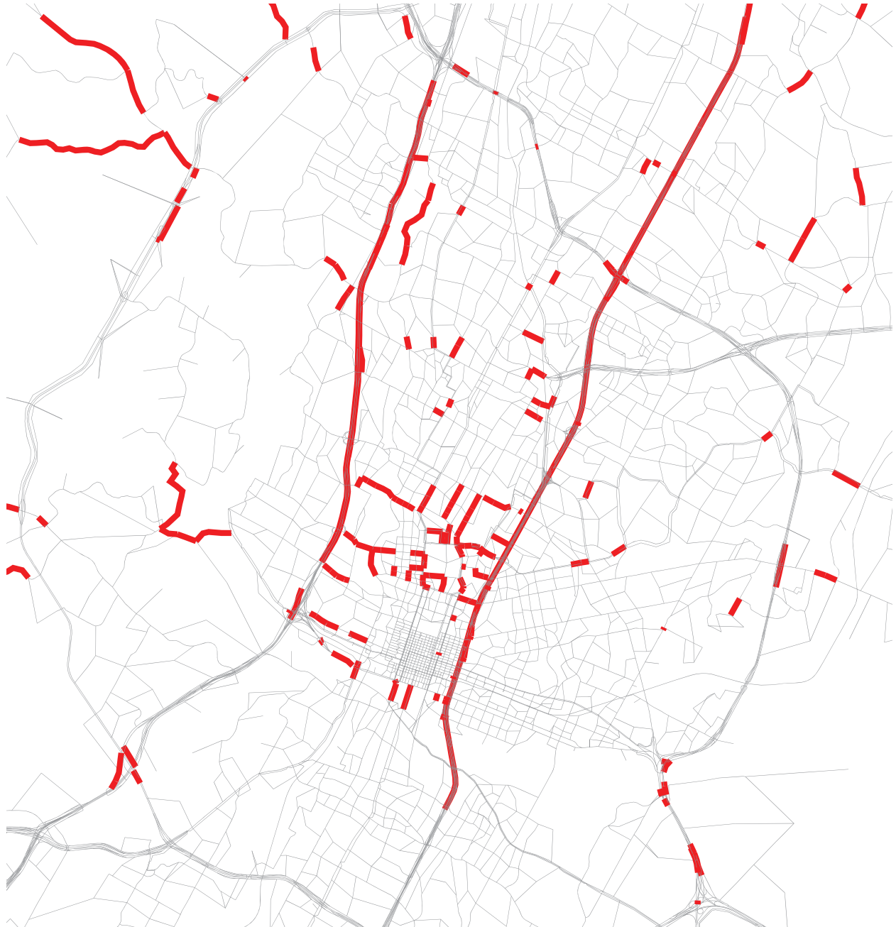
Figure 10: STA-Q Model 2045 Afternoon Peak Period Volume-to-Capacity Ratio Exceeding 1.1 (RED)
