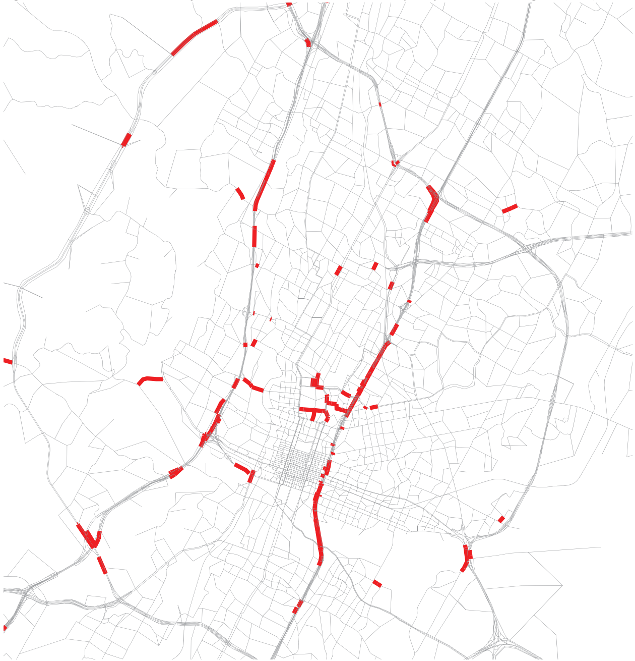
Figure 1: CAMPO 2015 Model Afternoon Peak Period Volume-to-Capacity Ratio Exceeding 1.1 (RED)
